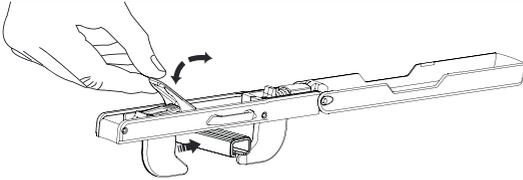
Stop ratcheting when both hooks meet roof rack
