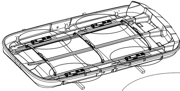
Attach the roof box to the roof racks on all four attachment point.
